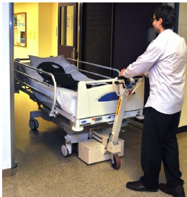
Figure 4: One of the subjects using the StaminaLift during a trial. The four 20 kg weight discs are placed evenly along the bed.
